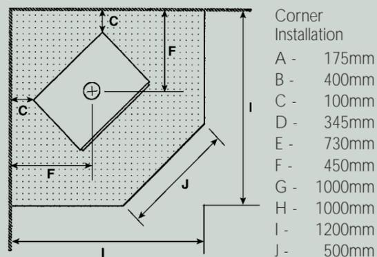
One 900mm length of heatshield must be fitted to the flue to achieve clearances to heat sensitive materials (measurements A B C D E F).
